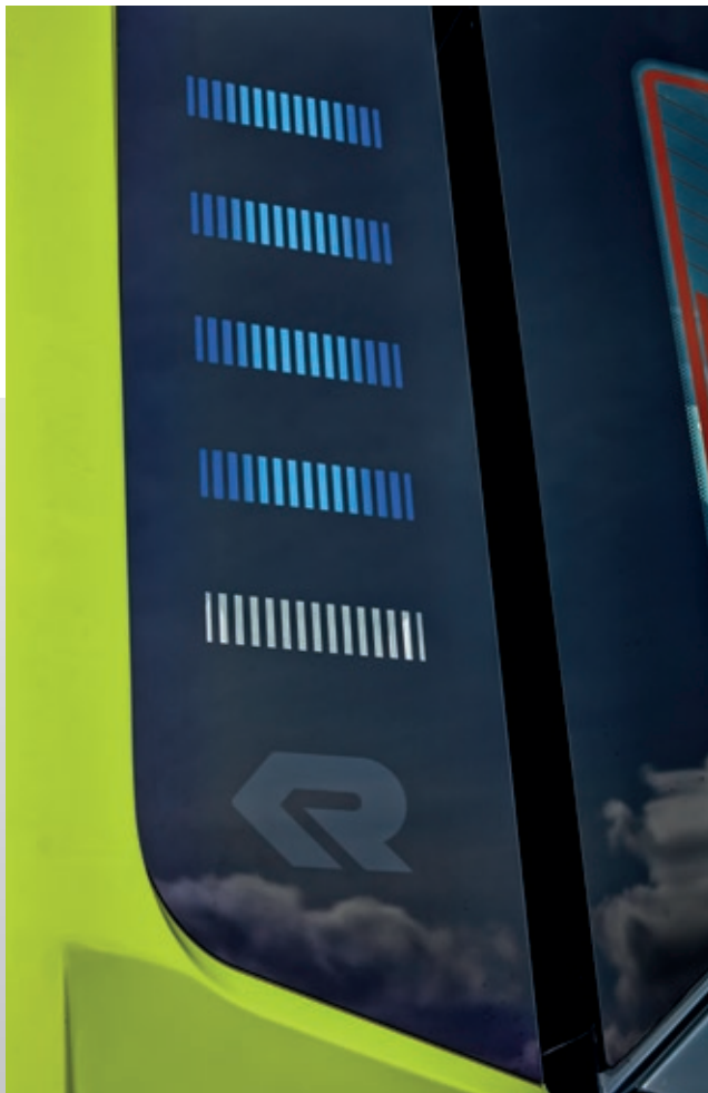
External tank indicator
