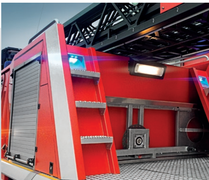
Completely new podium design (aluminum) with large toolbox behind the driving compartment.
